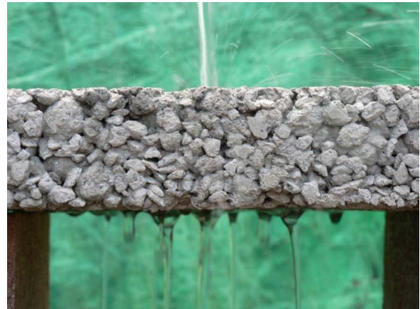
Pervious Concrete (TecEco, n.d.)
